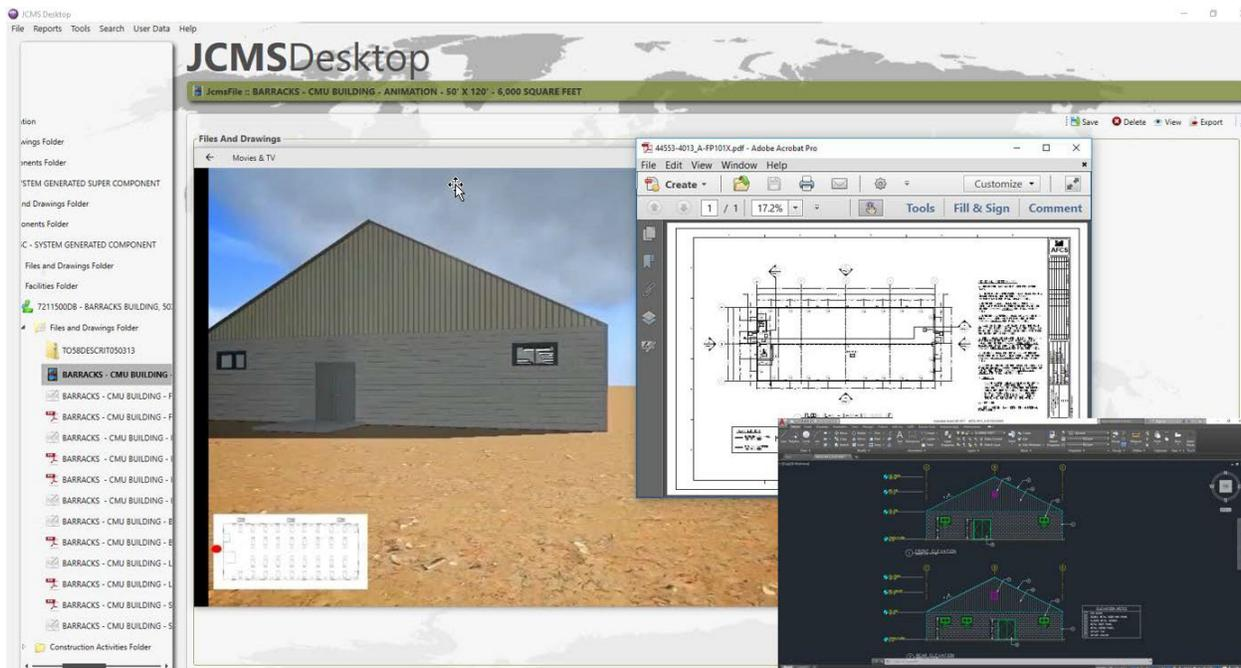
Screenshot of the JCMS application highlights some of the data produced and curated by the AFCS Program. A standard CMU barracks building is displayed in a 3D model walkthrough, construction quality .pdf plans, and editable 2D AutoCAD files.
